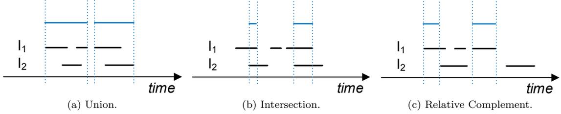
Fig. 4. A visual illustration of the three interval manipulation constructs of RTEC. In this example, there are two input fluent streams,  $I_1$  and  $I_2$ . The output of each interval manipulation construct is colored light blue.
