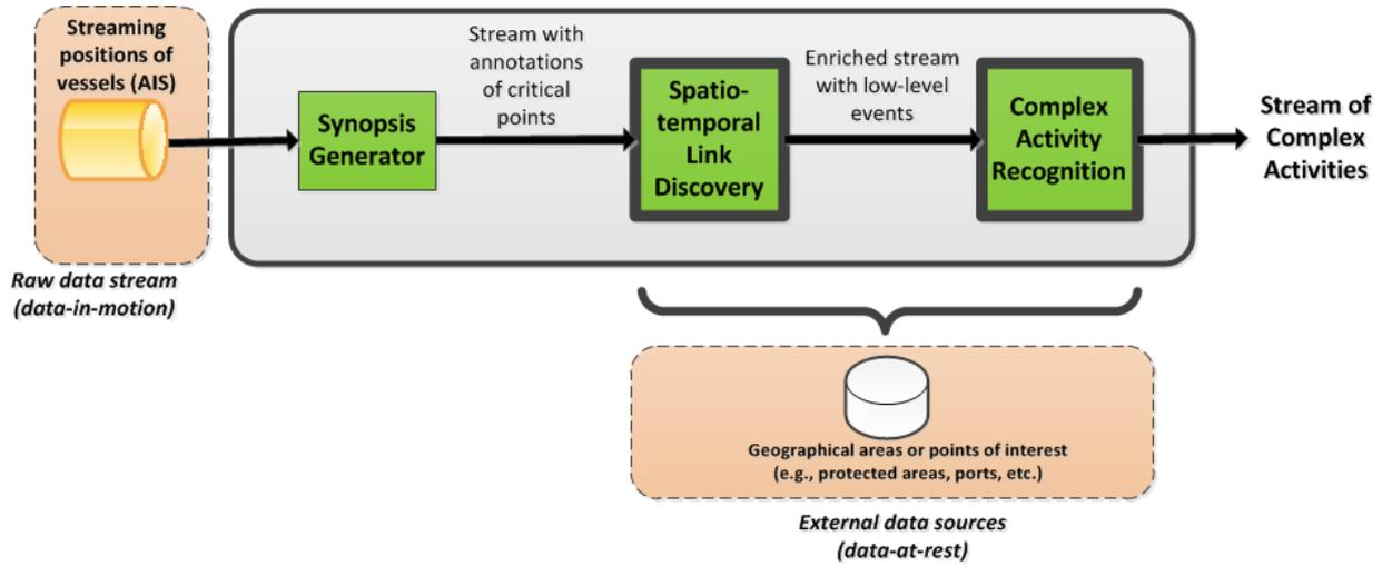
Fig. 1. The datAcron prototype architecture.
