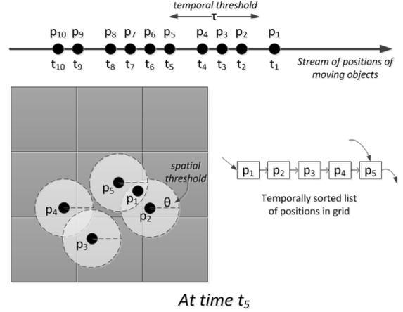
Fig. 3. Example of grid and bookkeeping structure for ‘nearby’ LD between positions of moving vessels.
