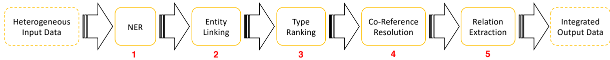
Fig. 1. The XI Pipeline goes through a series of five steps to integrate semi-structured or unstructured content leveraging a Knowledge Graph
